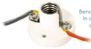
Bulb holder – Bend wire around screw in direction of turning when tightening
